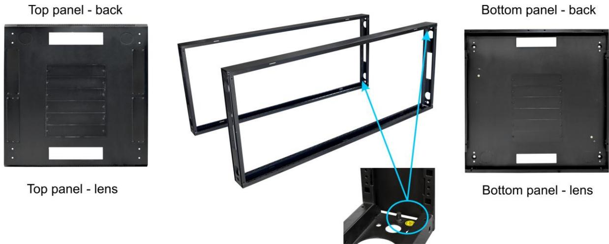
**5.2** Mount the top plate and bottom plate to the left and right frames of the RACK cabinet, respectively. Use M8x12 Head Cap Screws with M8 nuts (16pcs). Screw the cabinet **wheels** and **legs** to the bottom plate of the cabinet.
