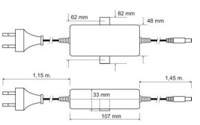
Fig.1. Dimension of power supply.
