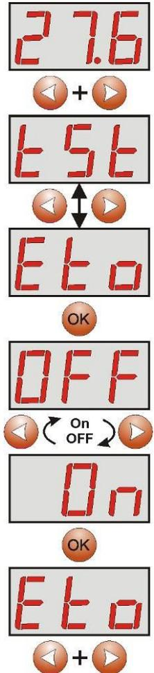
6.3.3. Setting the delay time for EPS output „EPS”
