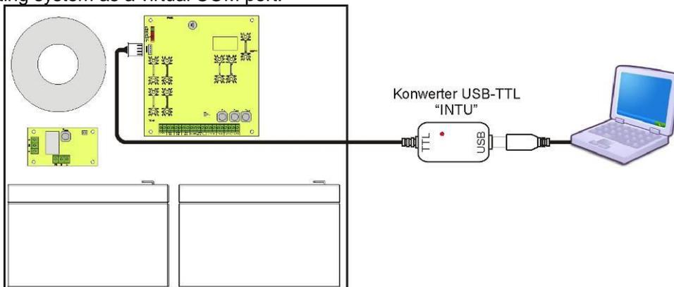
Fig. 15. USB-TTL communication using the USB-TTL „INTU” interface
