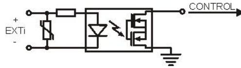
Fig. 11. Electrical diagram of the EXT IN input.
