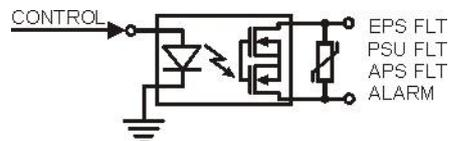
Fig. 10. Electrical diagram of technical outputs.
