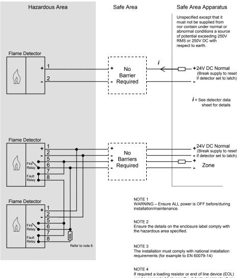
If required a loading resistor or end of line device (EOL) can be connected between the detector terminals of any circuit. The total power dissipation and temperature classes within the enclosure must not be exceeded, 30W - T6.
