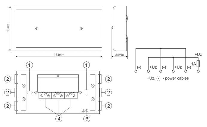
Fig.1. The junction box and wiring diagram.
