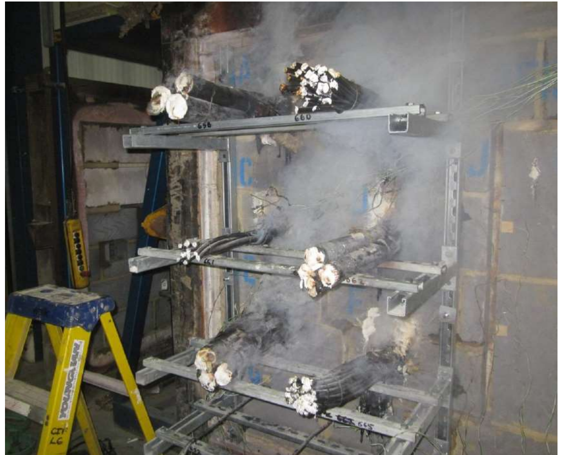
Picture shows a fire test after 2 hours at BM Trada in UK
